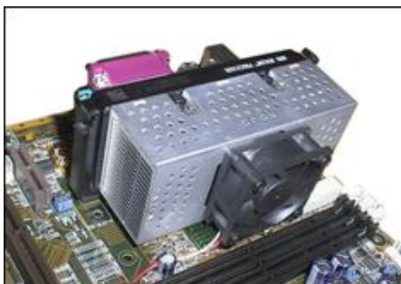
Figure 107. One of the first AMD Athlon processors, mounted in a Slot A socket. See the large cooling element.
