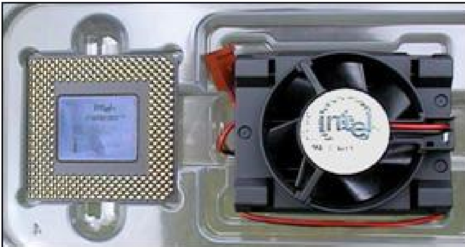
Fig. 36. A Celeron processor supplied in a box from Intel, with heat sink and fan.
