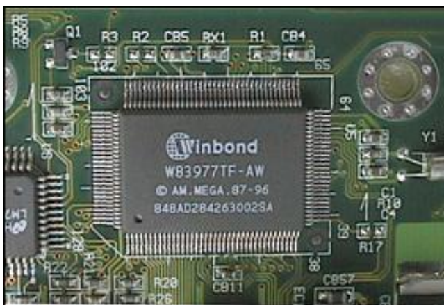
Figure 193. A super I/O controller from Winbond.
