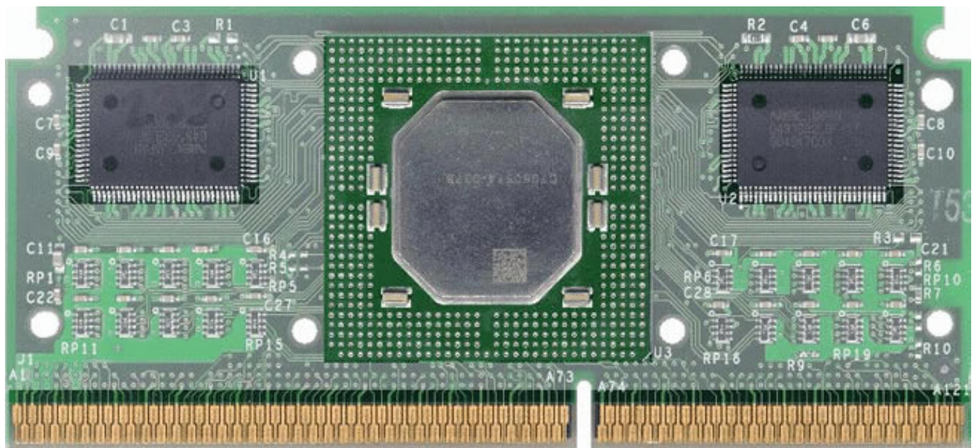
Fig. 71. An old Pentium II module. The CPU is mounted on a rectangular printed circuit board, together with the L2 cache, which is two chips here. The whole module is installed in a socket on the motherboard. But this design is no longer used.
