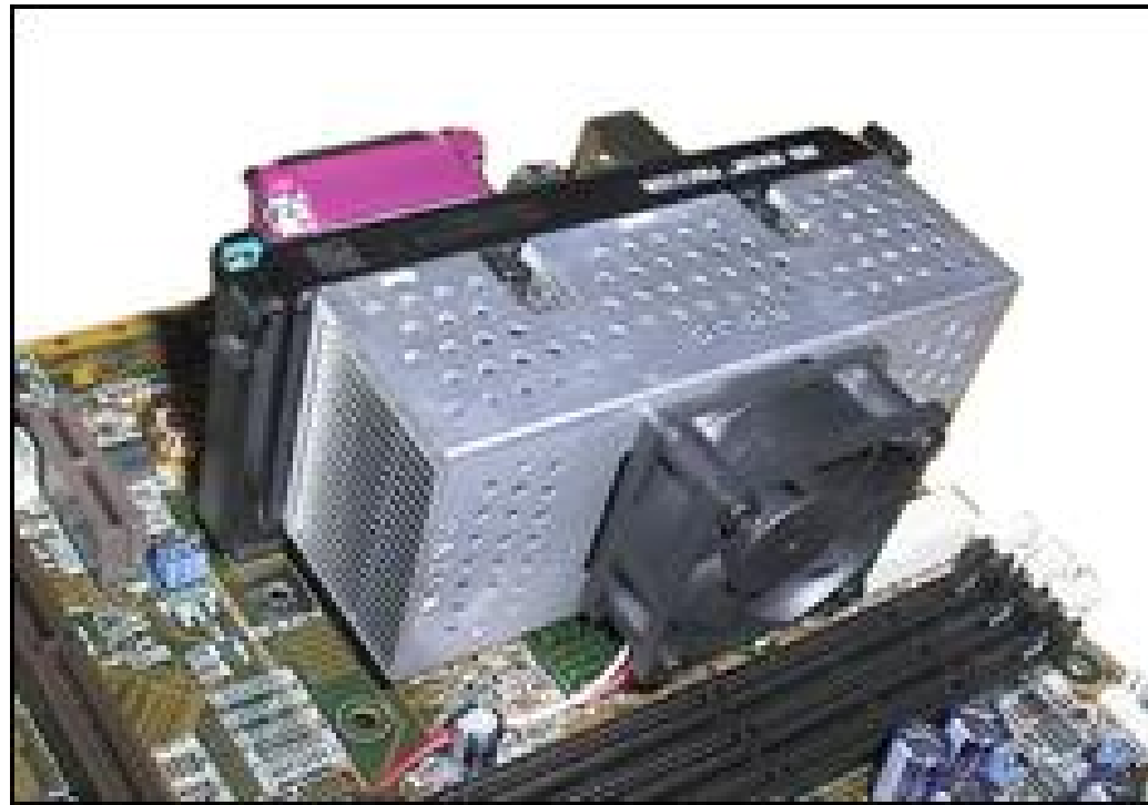
Fig. 107. One of the first AMD Athlon processors, mounted in a Slot A socket. See the large cooling element.
