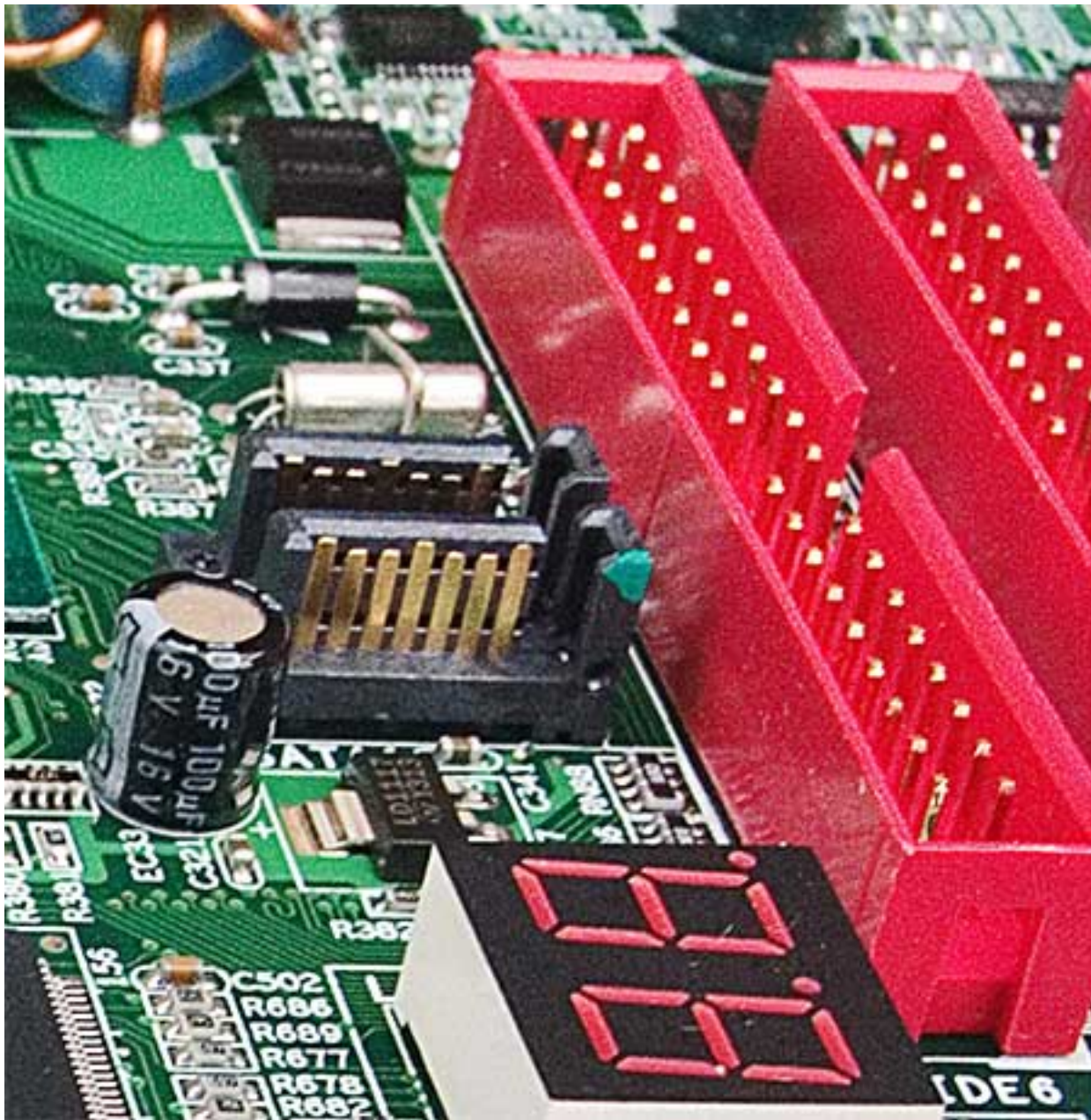
Figure 232. The small SATA connector is seen left to the bigger PATA-connector. This motherboard support both interfaces.
