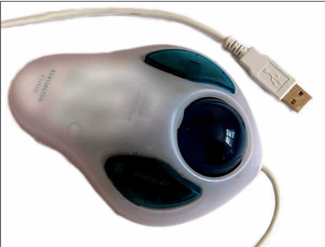
Figure 207. A USB-based trackball – actually designed for Macintosh computers, but works fine on PC's.
