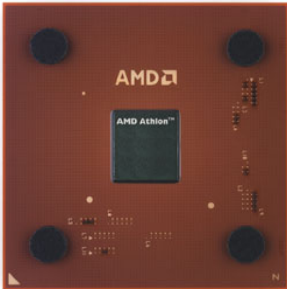
Fig. 33. The CPU circuit (the "die") can be seen in the middle of the chip (An AthlonXP shown close to actual size).
