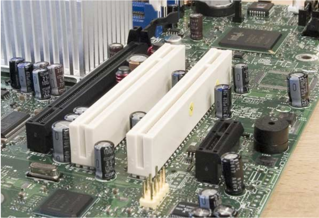
Figure 176. The two black slots are for PCI Express cards. To the left a 16X card for the graphics controller and to the right a smaller 1X slot. Inbetween you see two traditional PCI slots.
