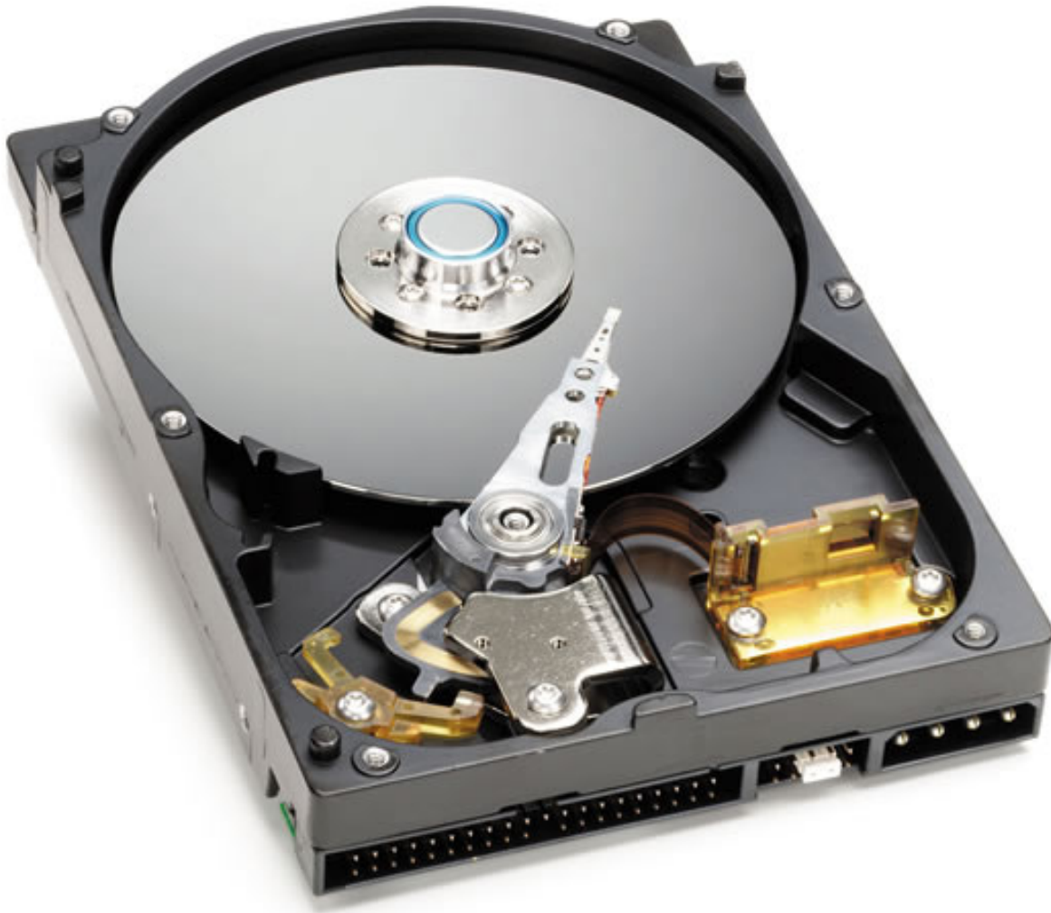
Figure 216. A peek inside the hard disk reveals the magnetic plates, which have a diameter of 3½ inches.
