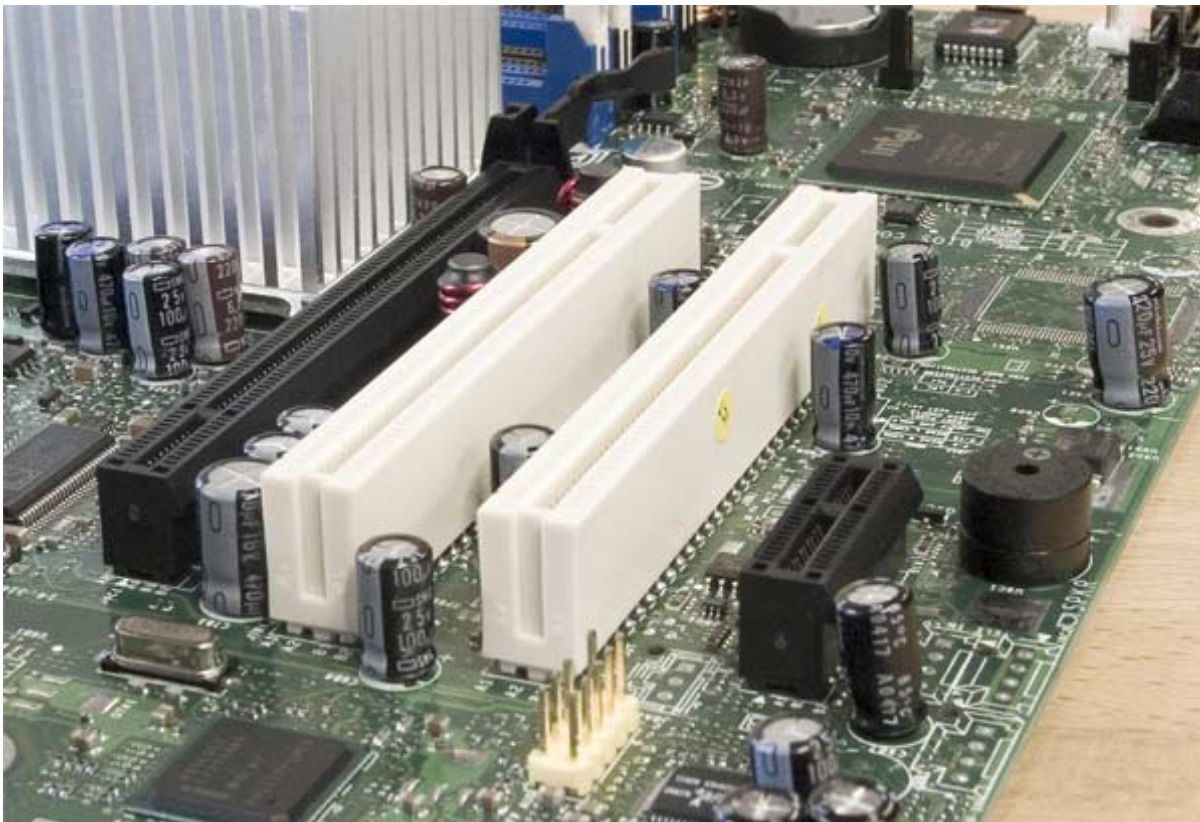
Figur 176. The two black slots are for PCI Express cards. To the left a 16X card for the graphics controller and to the right a smaller 1X slot. Inbetween you see two traditional PCI slots.
