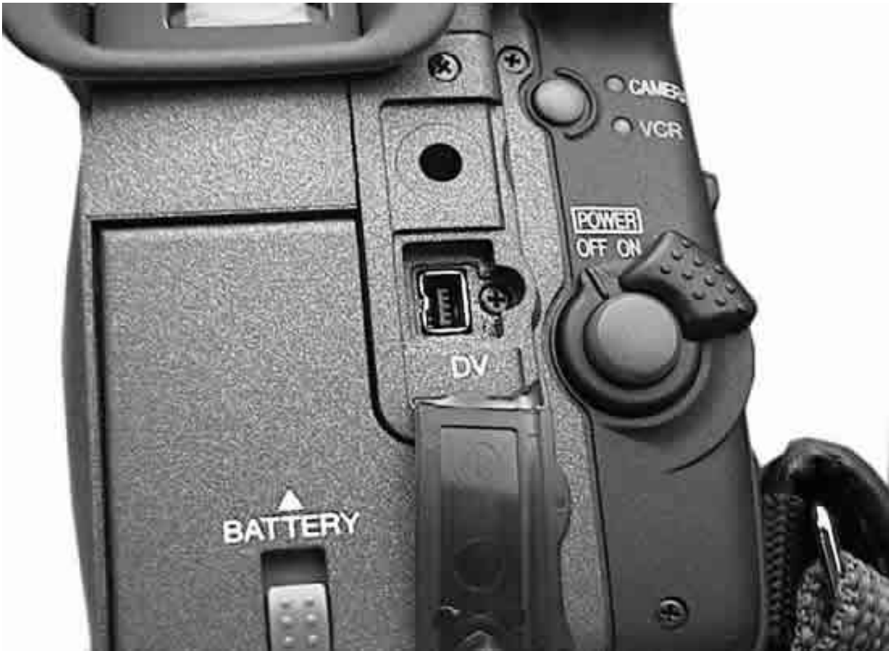
Figure 211. In the middle of the picture you can see the small DV connector on this digital video recorder.
