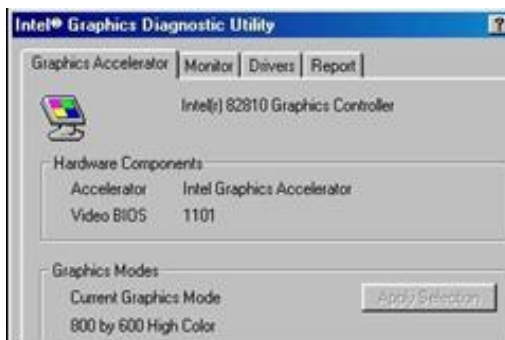
Figure 52. This PC uses a video card which is built into the Intel i810 chipset.
