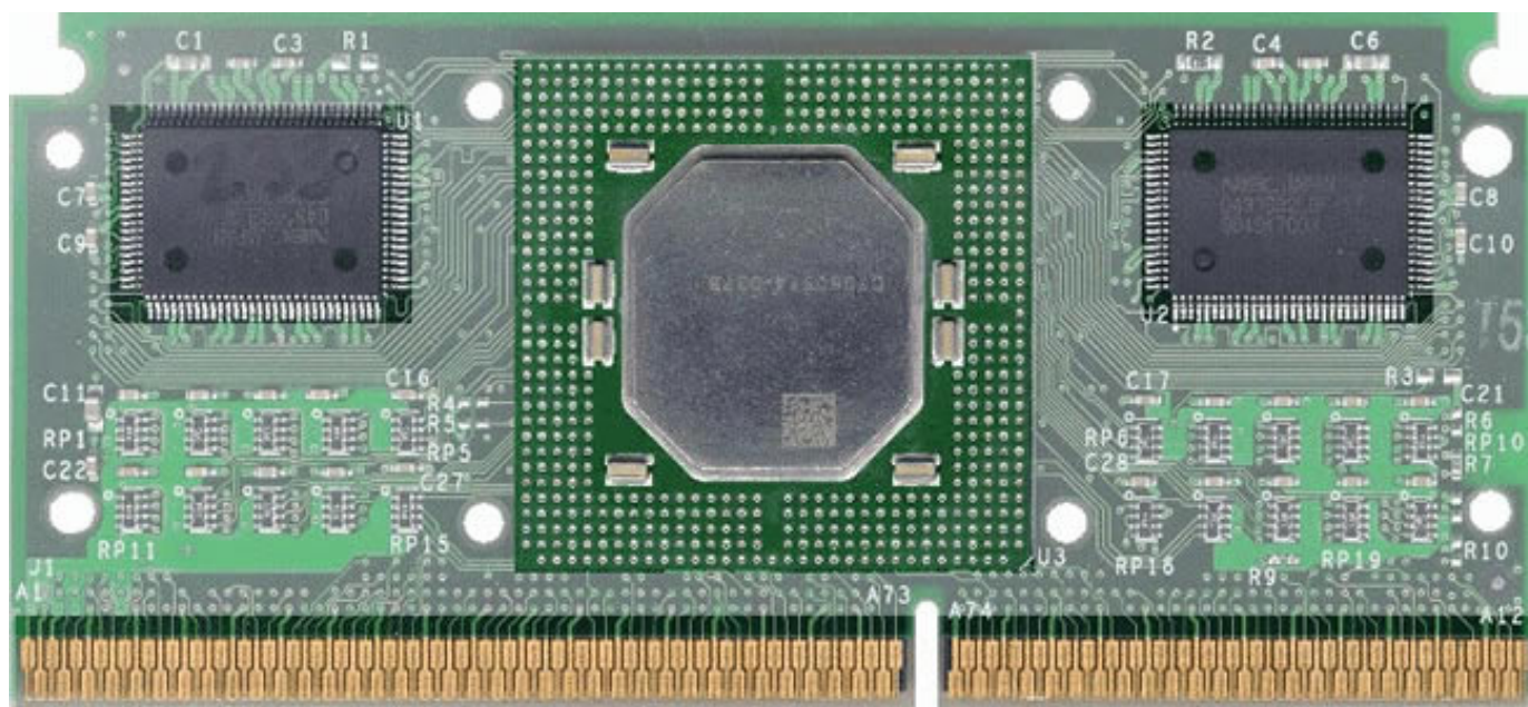
Figure 71. An old Pentium II module. The CPU is mounted on a rectangular printed circuit board, together with the L2 cache, which is two chips here. The whole module is installed in a socket on the motherboard. But this design is no longer used.
