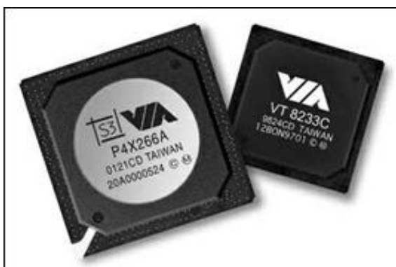
Figure 49. The two chips which make up a typical chipset. Here we have VIA's model P4X266A, which was used in early motherboards for Pentium 4 processors.
