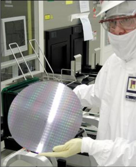
Figur Figure 65. A technician from Intel holding a wafer. This slice of silicon contains hundreds of tiny processor cores, which end up as CPU's in everyday PC's.
