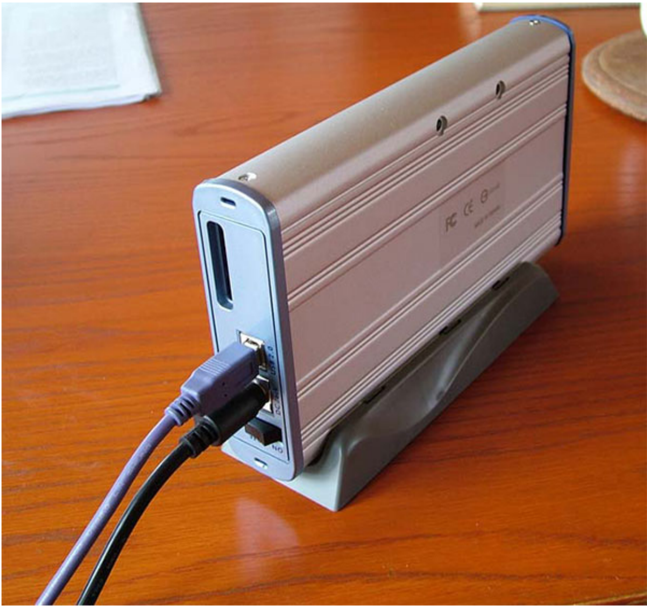
Figure 208. An in-expensive USB 2.0-based hard disk box. You can use any old hard disk in it. Great for backup!
