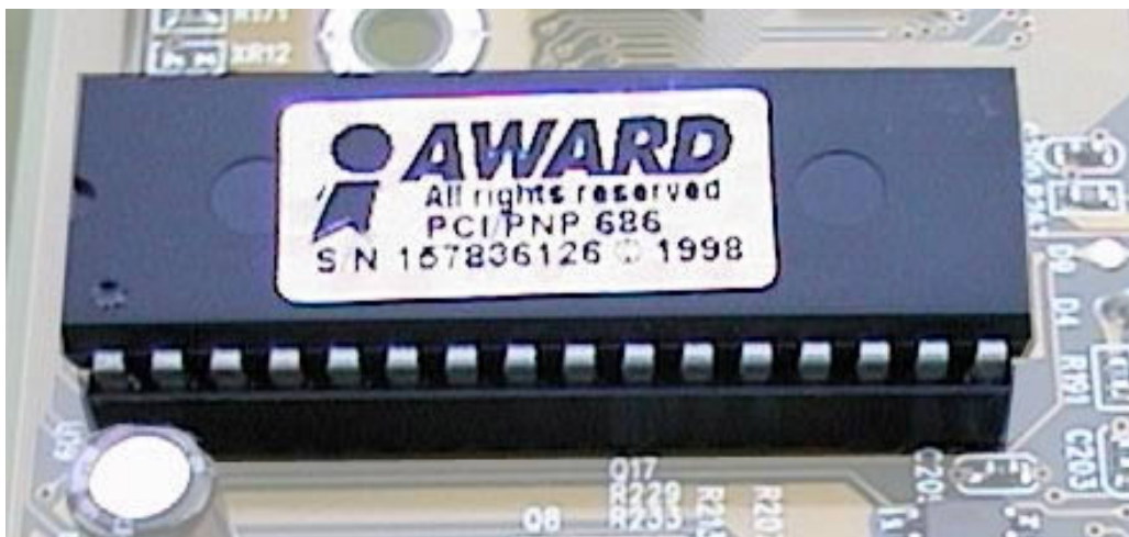
Figure 233. A ROM circuit containing Award BIOS (typically 1 or 2 MB of data).
