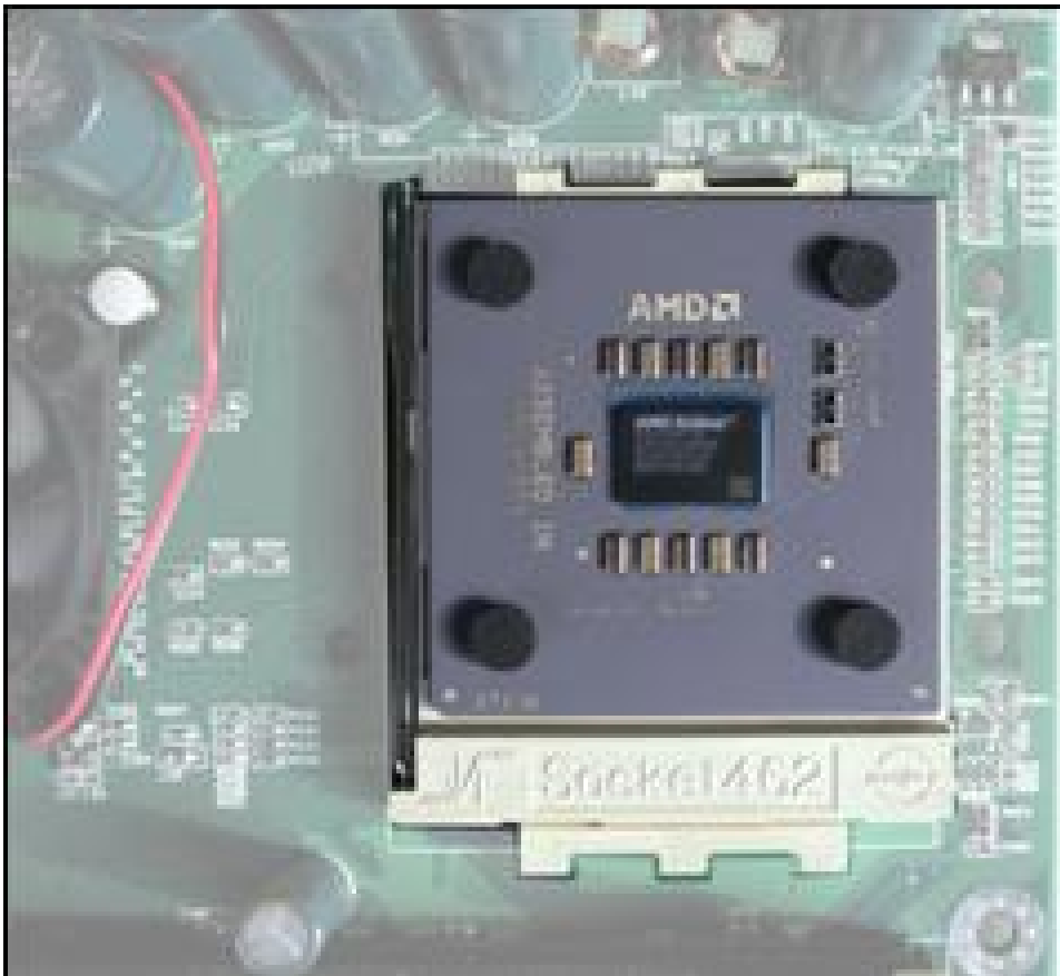
Fig. 38. A CPU is shown here without a cooling fan. It is mounted in a small socket which it clicks into without needing any tools.
