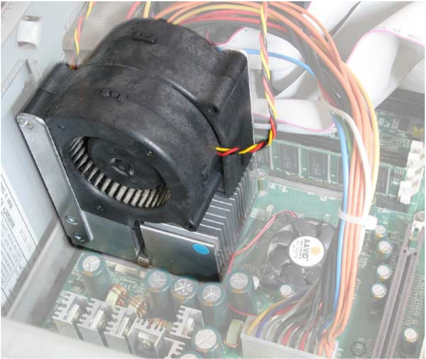
Figur 124. A gigantic cooler with two fans and pure silver contact surfaces. Silverado, a German product which is used for overclocking CPU's.
