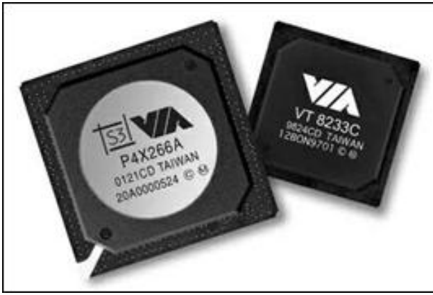
Fig. 49. The two chips which make up a typical chipset. Here we have VIA's model P4X266A, which was used in early motherboards for Pentium 4 processors.
