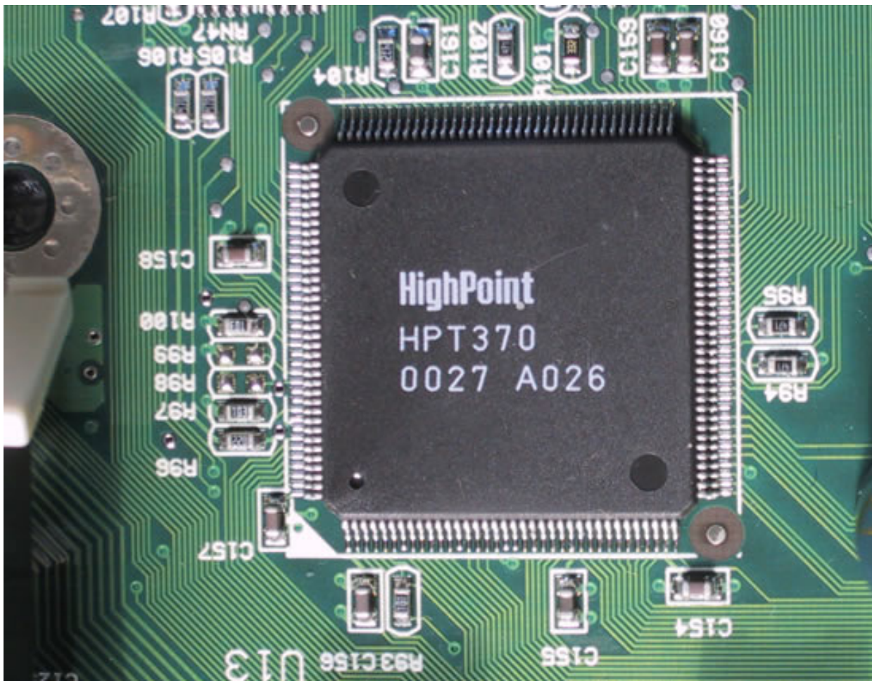
Figure 228. An ATA-RAID controller which is integrated into the motherboard.
