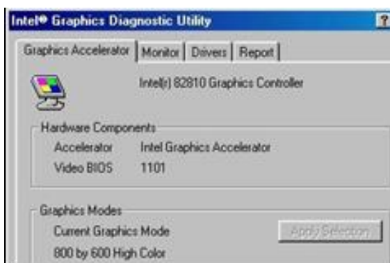
Fig. 52. This PC uses a video card which is built into the Intel i810 chipset.
