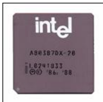
Figure 94. A “separate” FPU, Intel's 80387 from 1986.
