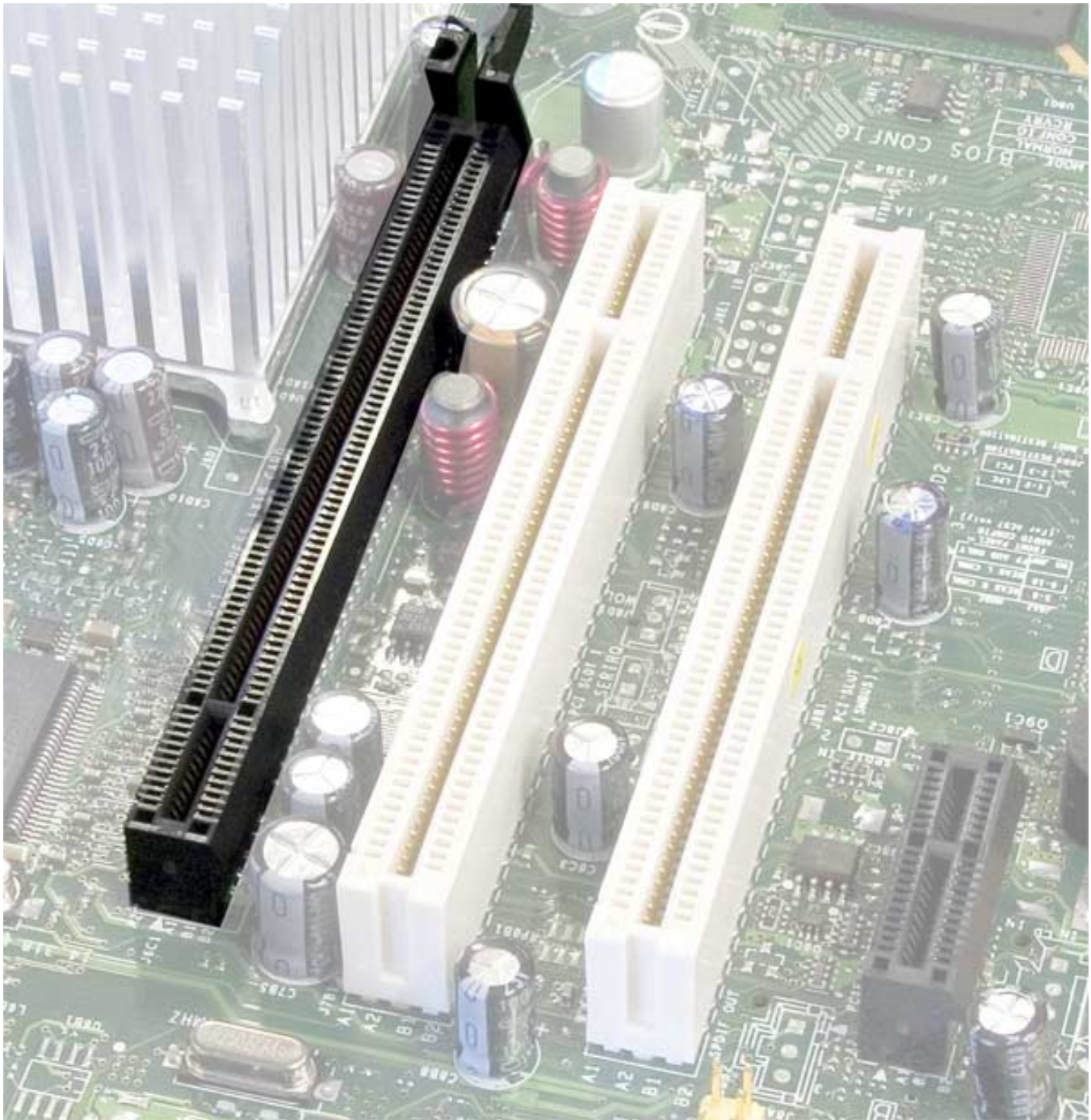
Figur 156. The black PCI Express X16-slot to the left is for the video card.
