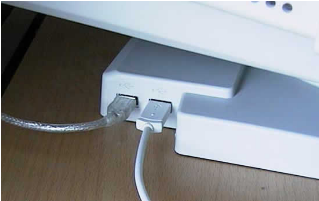
Figure 209. This screen has a built-in USB hub in its base. That means that a further four USB devices can be connected to the screen, which is itself connected to the PC's USB connector.
