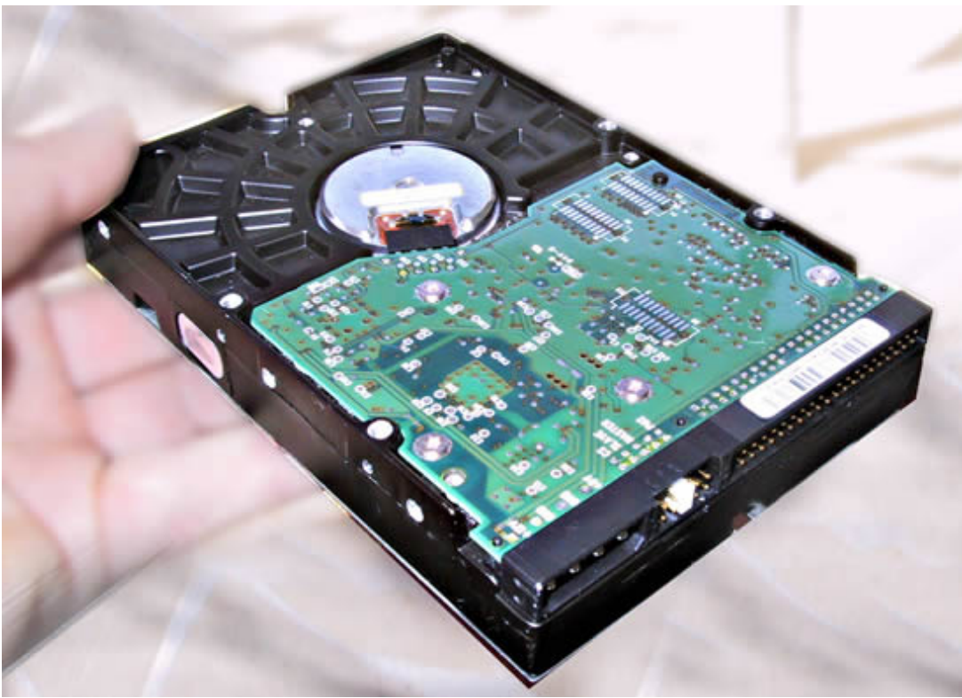
Fig. 21. Underneath the hard disk you can see a small printed circuit board. This incorporates the controller functions which work together with the corresponding controller in the PC's motherboard.
