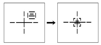
In addition, for additional indication of the "AUTOMATIC TRACKING" mode, a symbol for the presence of automatic target tracking 8 is displayed in the ISM optical channel (Figure ).
