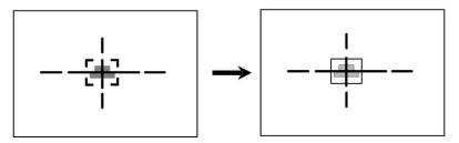
When operating in the "INERTIAL TRACKING" mode, the BCOI provides automatic tracking of the predicted position of the captured target according to the parameters recorded at the time of interruption of optical communication with the target (characteristics of the target image, speed and direction of its movement are remembered).
