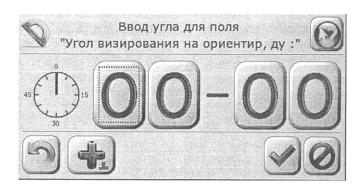
At the top of the window for entering numerical values there are keys for controlling step-by-step changes in values and a scale informing about the range of permissible values and the current value of the entered value.
